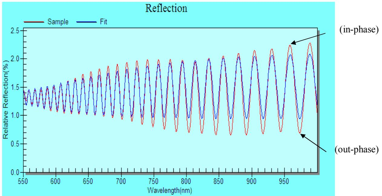
It shows that the refractive ratio of film will be changed periodically with respect to  $1/\text{wavelength}$ . The thicker film will generate the amplitude change with higher frequency within fixed wavelength range. the refractive ratio of film will be changed periodically with respect to  $1/\text{wavelength}$ . The thinner film will generate the amplitude change with lower frequency within the same wavelength range.
